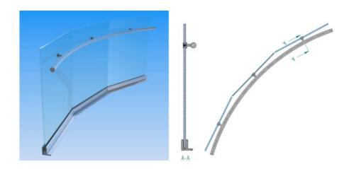
**Alternative 2** > facetted glass with wide slot in slotted handrail.
